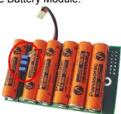
Install the Battery Module on the RTCU unit. First align the Battery Module on top of
