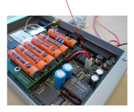
Leaving the power-connector disconnected will relatively fast drain the on-board Lithium battery. The on-board Lithium battery is used to maintain the Real-time clock, GPS almanac and is required for power-down to work.
