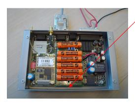
4. Connect the power plug to the white connector on the RTCU unit.
