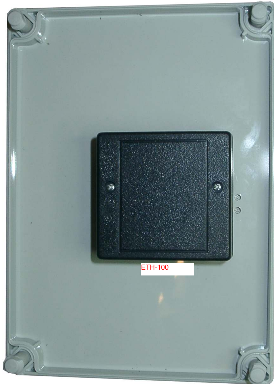
The ETH-100 Ethernet module mounted in the lid of the RTCU A9 unit.
