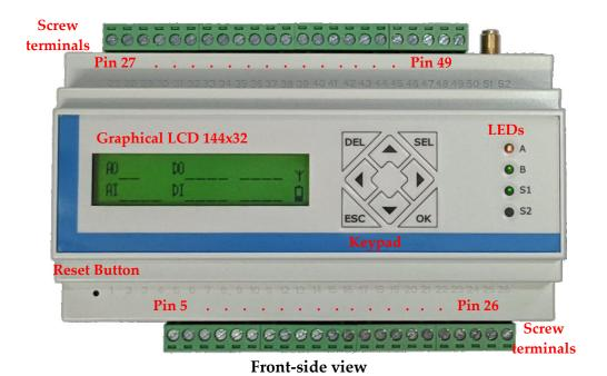
The pluggable screw terminals on the top and bottom sides of the LX4 pro are used to make connections to external equipment.
