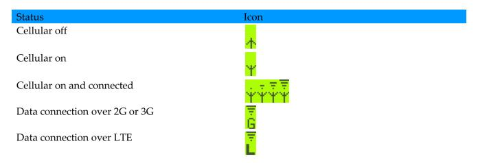
The cellular signal level is indicated with 4 bars – also known from many mobile phones. One bar means low signal strength, and four bars represent high signal strength. No signal strength bars indicate that the cellular interface is powered up but is not connected to the network.
