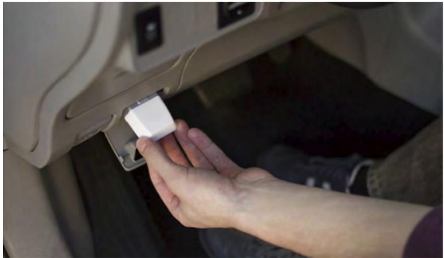
*Small dongle inserted in an OBD port in a vehicle.*
