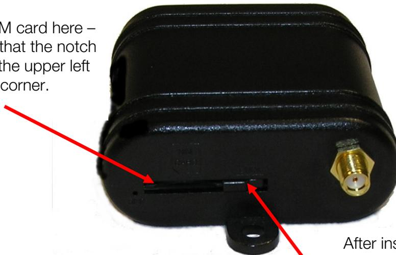
After inserting the SIM card, you MUST move the SIM lock switch to the left. If the lock is open, there will not be power to the SIM.
