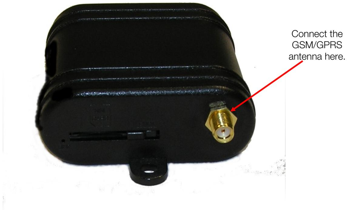
Figure 6 GSM/GPRS SA-G+ Connecting the Antenna
