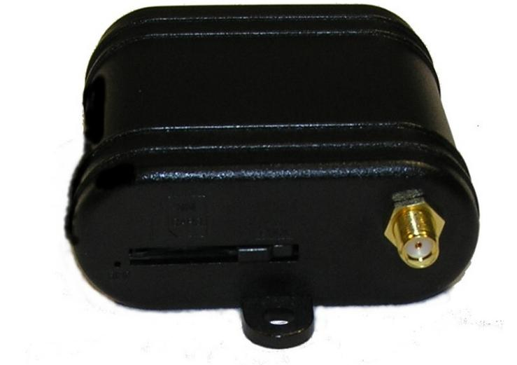
Figure 1 - Front view of GSM/GPRS SA-G+ modem.
