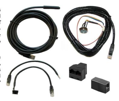
The modular 1-Wire network can easily be designed and implemented using standard of the shelf RJ-45 cables, splitters and/or combiners allowing multi device network to be configured to meet the requirements of the application / installation. Several 1-Wire devices such as temperature sensors and ID-Button readers can be connected to the same network.
