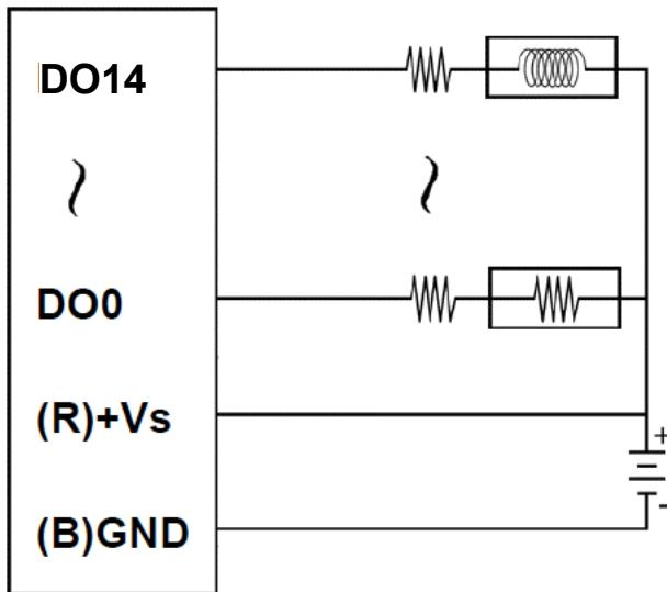
*Please note that when connecting inductive load to the digital outputs a diode needed to prevent counter EMF.*
