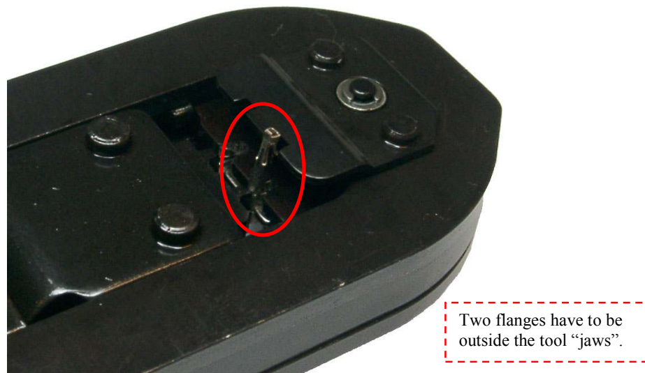
Figure 3 – Back view of crimp contact placement.
