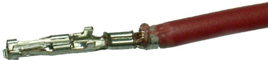
Figure 5 – Correct crimped contact.
