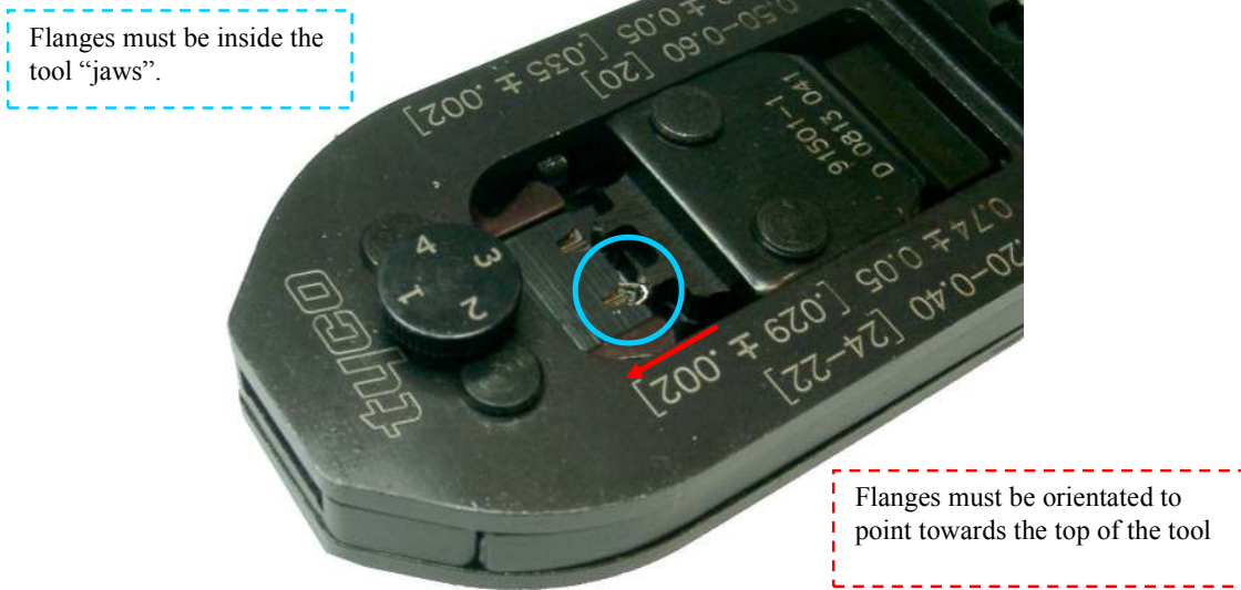
Figure 2 – Front view of crimp contact placement.
